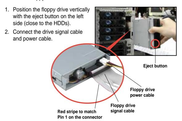
3. Carefully push the drive into the bay until the drive cage fits the front edge of the bay.
